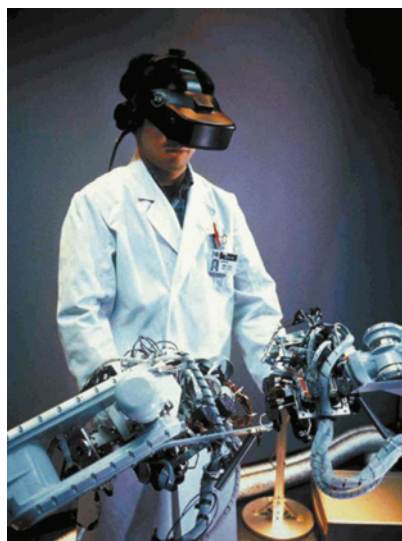
Fig. 4. Synthetic reality allows surgery to be realistically planned, rehearsed and/or remotely conducted using highly interactive visualization, haptic and robotic controls, such as is possible with this two-handed haptic and 3-D visualization system (courtesy of Dr. Naoki Suzuki, Jikei University, Tokyo).
